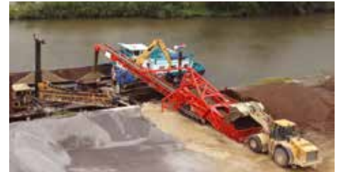
Telestack Mobile Truck Unloader loading a barge directly from wheel loaders
